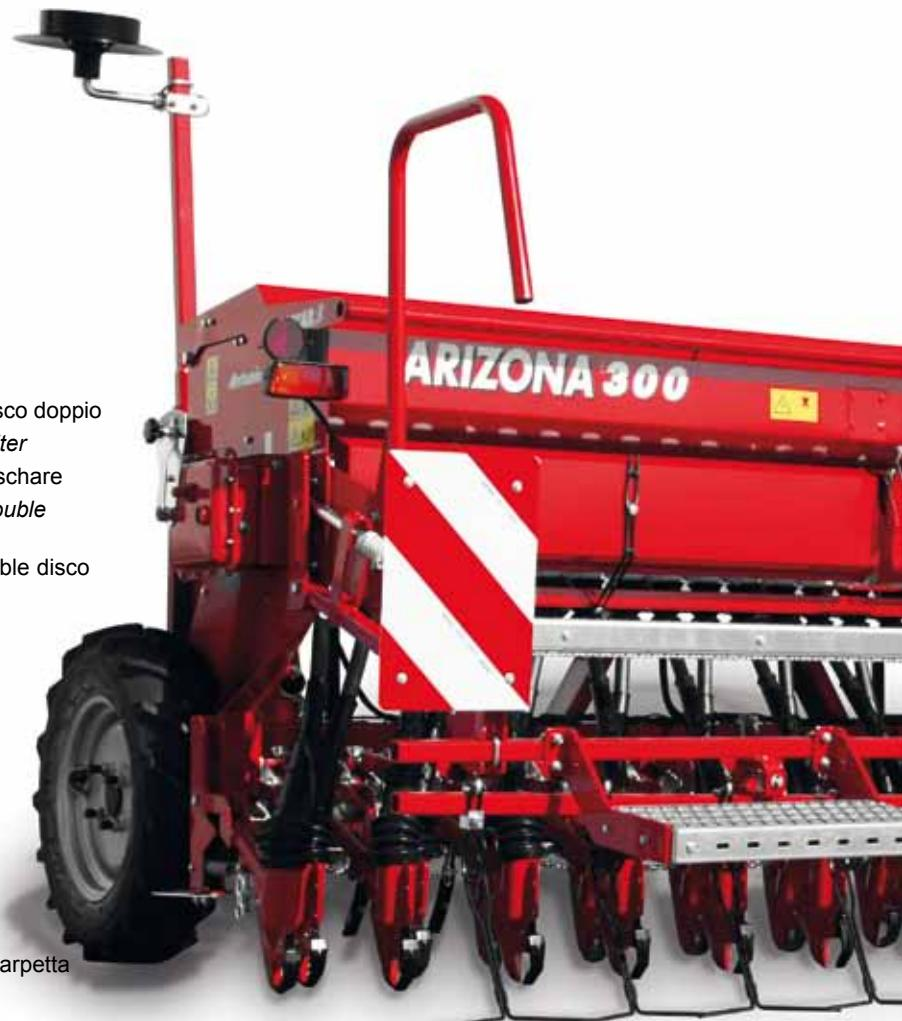
**EN** ARIZONA is a mechanical seed drill for cereals and small seeds. It is equipped with a hopper of big dimension for the better operating range. The machine has a continuous oil immersed gear box for a precise and fast seed quantity regulation. The volume grooved batchers guarantee a regular seed division for all the rows and uniform distribution even if operating in areas with steep slopes. The machine is available with suffolk coulters, coulters and double discs.
